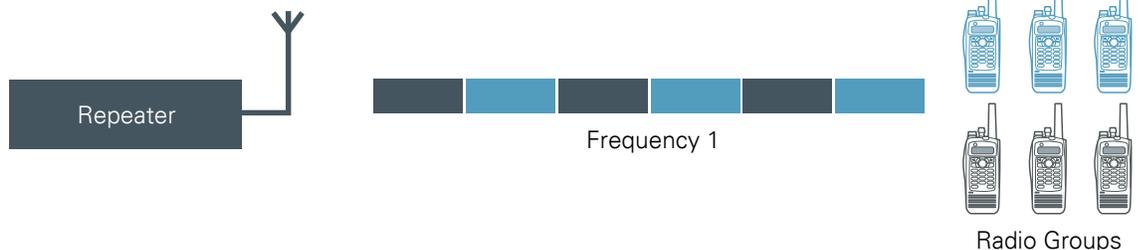
TDMA-based systems also offer the flexibility to adapt as new applications emerge to make additional use of the two time slots — preserving initial investments while providing an open path to future usage models for digital two-way radio. For example, the future roadmap for two-slot TDMA applications includes the ability to temporarily combine slots for increased data rates, or to use both slots together to enable full-duplex private calls.
